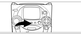
When the VOCAL feature is activated, the vocals on a multiplex recording are muted as soon as the singer begins singing into the microphone. When the singer stops singing, the vocals are automatically unmuted. Adjust the AUTO VOCAL control for the best balance between playback and microphone levels. **IMPORTANT:** This feature only works with multiplex CDs.
